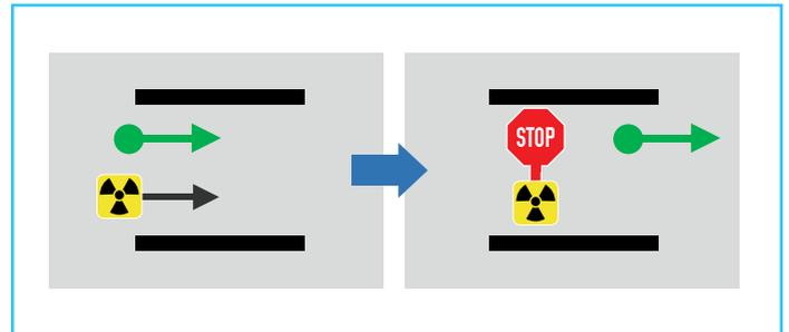
**Figure 3.** Source remaining inside the monitor
