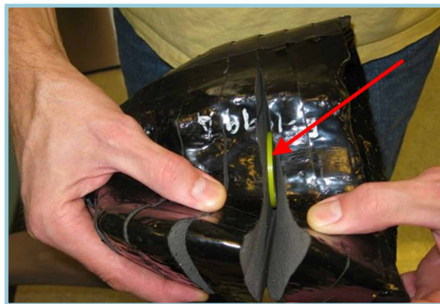
Figure 4 Sectioned lungs with radioactive disk source
