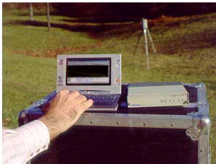
Figure 2 The InInspector 2000 MCA with its Laptop Control and Analysis Computer and Germanium Detector in a Big MAC Cryostat.
