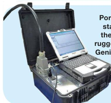
Portable acquisition station containing the Lynx DSP and a ruggedized laptop with Genie™ 2000 software
