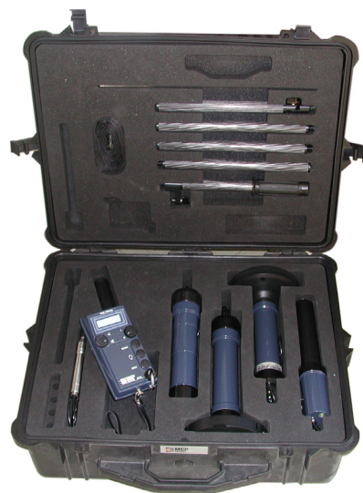
Carrying case with external: beta/gamma probe, alpha 125 probe, X probe, TGS probe and pencil probe.
