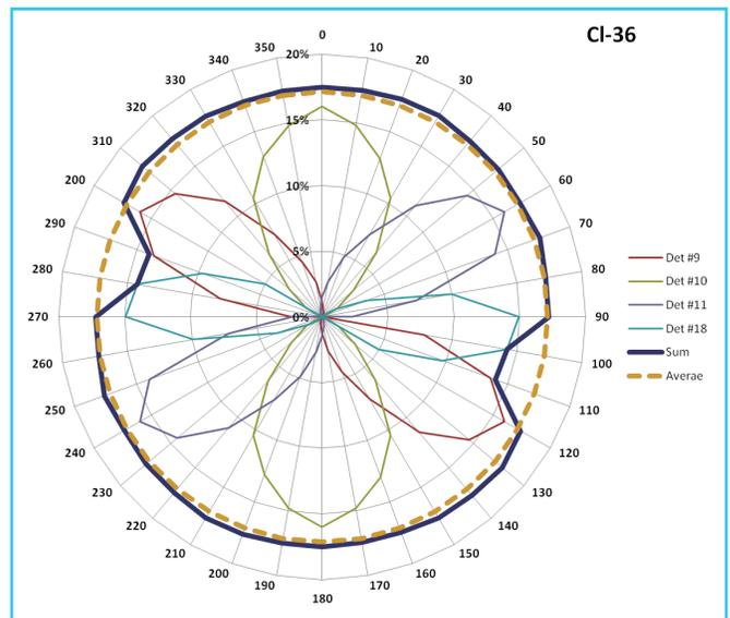
Argos-3/-5PAB Horizontal Scan Efficiency for <sup>36</sup>Cl, IEC 61098 Phantom test 5 cm from center detector.
