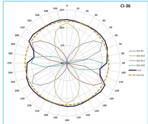
Argos-3/-5PBG Horizontal Scan Efficiency for <sup>36</sup>Cl, IEC 61098 Phantom test 5 cm from center detector.
