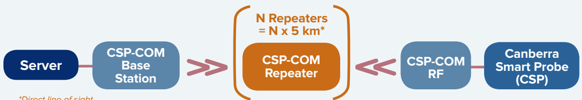
Figure 1: CSP-COM RF configuration with Base Station-Repeater.
