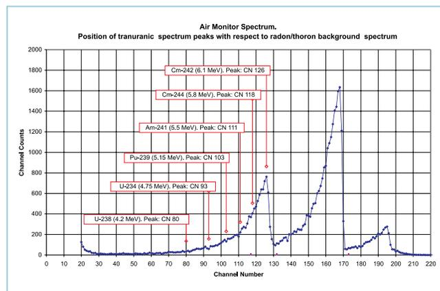
Figure 1: Spectrum showing radon/thoron interference and transuranic peaks.
