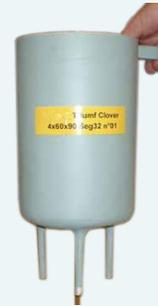
LN<sub>2</sub> filling funnel for manual filling in vertical position
