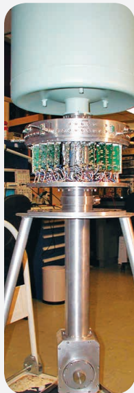
45-channel segmented Si(Li) detector within a dedicated LN 2 cryostat cooled.
