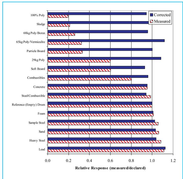
Figure 3. Typical AAS correction results for the IWAS counter for a series of homogeneous and non-homogeneous matrix drums with a simulated uniform source distribution. The uncorrected response is reported as much as a factor of five too low while the corrected response has a standard deviation of only a few percent.
