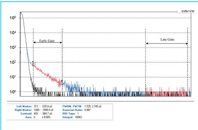
Figure 4. Time response of the Fast Neutron Detector Packages for a zero matrix drum. The upper curve shows the response for a 1 gram <sup>235</sup>U source and the lower for a drum with no fissile material.
