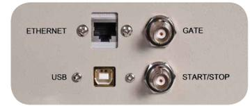
The cabling is minimal: two BNC cables to connect to the HPGe detector's Lynx DSA and an Ethernet and USB cable, one of which is used to interface to a Genie or Apex computer. This cable also powers the guard detector. Power-over-Ethernet (PoE) is required if the Ethernet interface is used, and a PoE single port injector is provided for this purpose.
