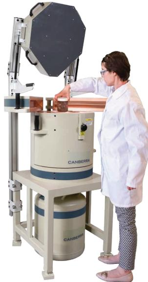
Each of the mentioned models includes the guard detector with built in electronics, appropriate mounting hardware (lid or frame), cabling and a software application compatible with Genie 2000 and Apex-Gamma software for setting up and managing operation of the system.
