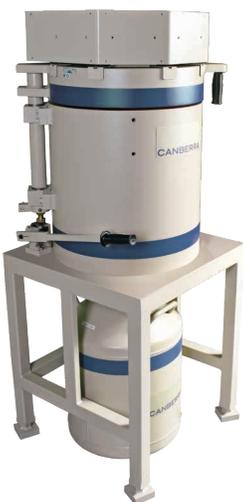
The Model CV SYSTEM-LM fits directly on model 737, 747, 747E and 777 shields or most any shield with a solid, circular lid having a diameter of 50.8 or 55.9 cm (20 or 22 in.).
