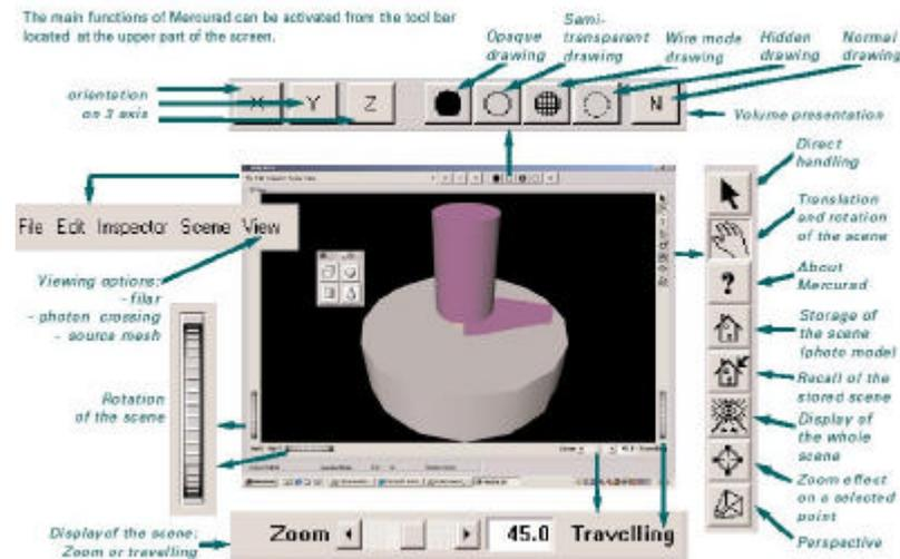
Figure 5 : Illustration of the scene manipulation tools in MERCURAD
