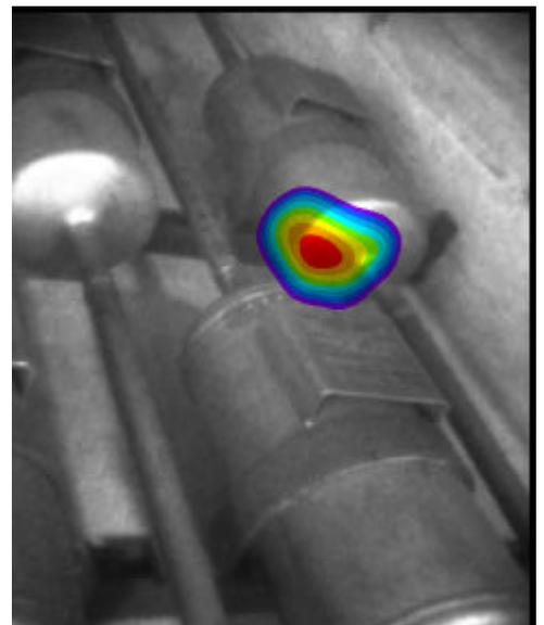
Figure 7 : CARTOGAM view showing a hot spot
