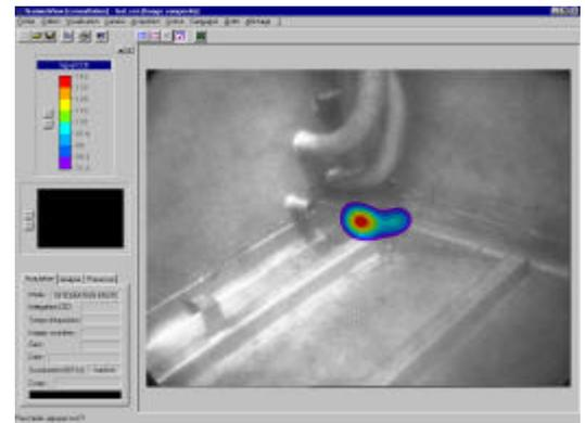
Figure 2 : CARTOGAM view with gamma and video images superimposed showing contamination near the discharge opening of a tank
