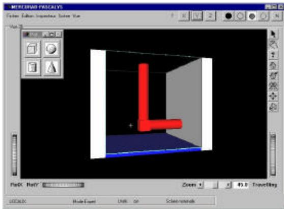
The calculated activity is used to create with MERCURAD a model of the item to be dismantled in order to calculate dose-rate during operation for job optimizing.
