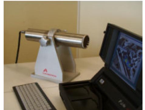
Figure 1 : CARTOGAM detector head, with portable stand and controlling PC
