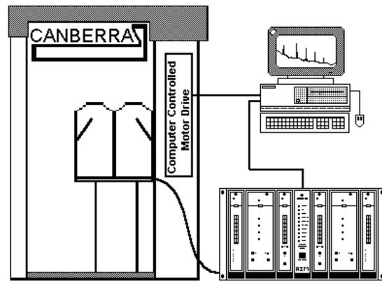
FIGURE 1 - ACCUSCAN-II with Dual HPGE Detectors
