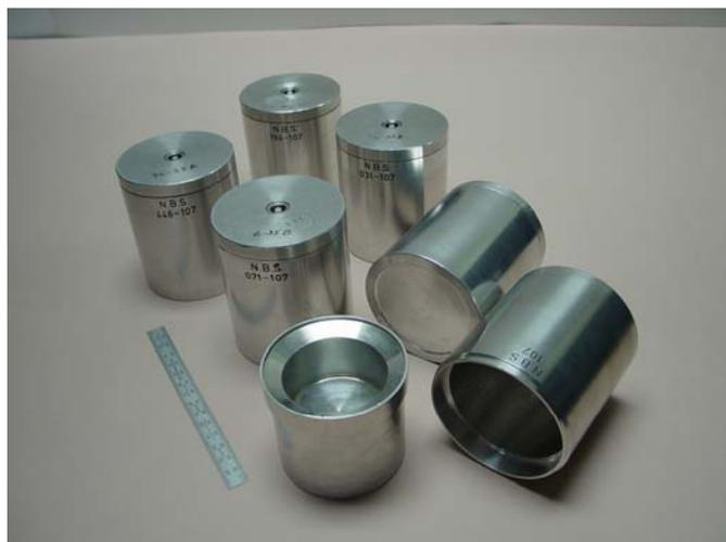
**Figure 2 Photograph of the NBS-SRM-969 standards**
