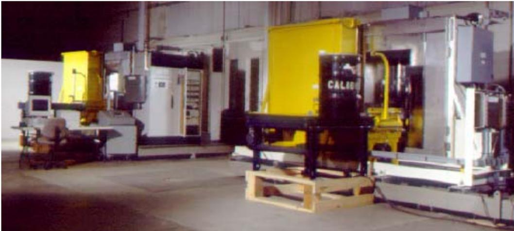
**Figure 1 Two IWAS units undergoing calibration. The HRGS detectors are out of view on the left hand side of each chamber.**
