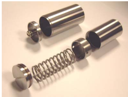
Figure 1. Encapsulation details of the AE4043 items. The inner capsule assembly (shown in the foreground) fits into the outer container (shown top).
