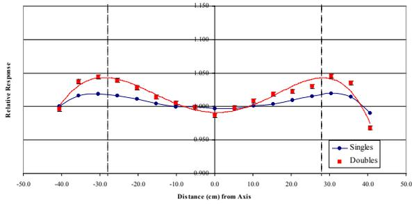
• Figure 7: Measured response for the X-axis, illustrating along the major extent of the hexagon. The dips at the extreme edges of the counter are due to the dead effects of the corner.
