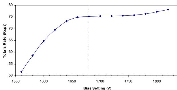
• Figure 4: High voltage plateau for the HNMC. Optimal HV setting is 1740 volts.
