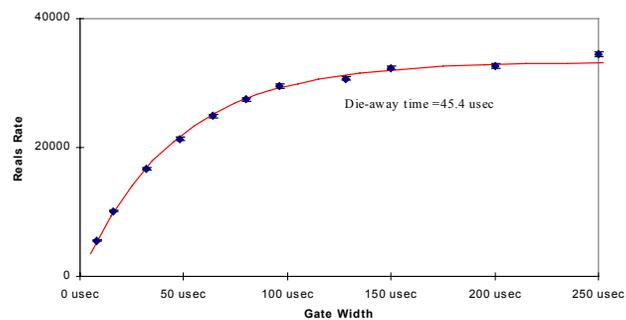
• Figure 5: Reals rate vs. gate width setting used to determine the die-away time of the counter.
