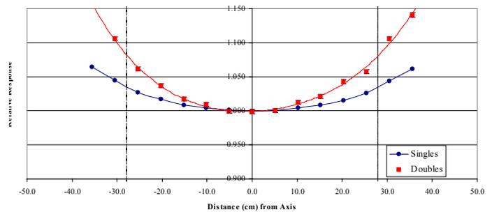
• Figure 8: Measured response for the Y-axis, illustrating the response profile along the minor extent of the hexagon.
