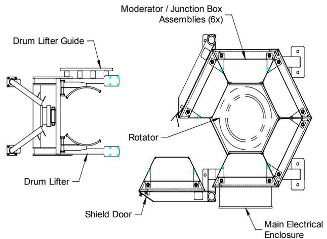
• Figure 3: Top view of the counter with the drum lifter shown.
