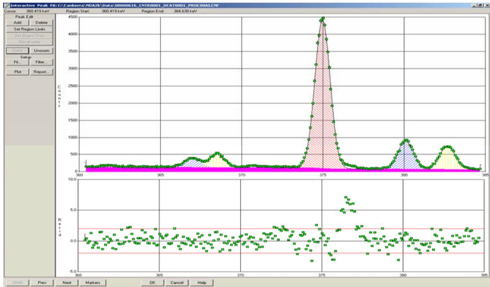
**Figure 1a: Spectral region showing overlap of Pa-233 and Pu-239 gamma ray peaks. Note the large positive residual at the bottom of the figure, showing the location of the unresolved 375.45 keV peak.**
