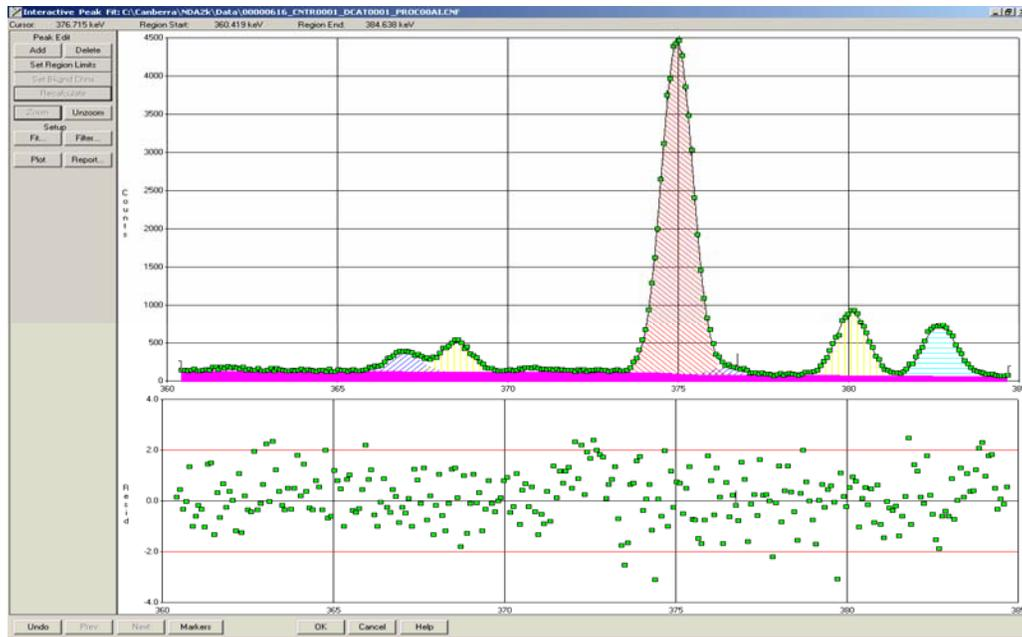
**Figure 1b: The same spectral region, showing addition of the missing peak at 375.45 keV, and the improved residual plot.**
