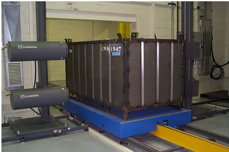
Figure 1. Photograph of a standard Canberra Modular Gamma Box Counter installed at a customer site. In this case this system used two pillars with 2 shielded HPGe detectors on each side of the crate. The crate is scanned through the counter as it moves from one process area to another. The distance between detector and crate is adjustable to allow the system to be used with higher exposure rate containers.
