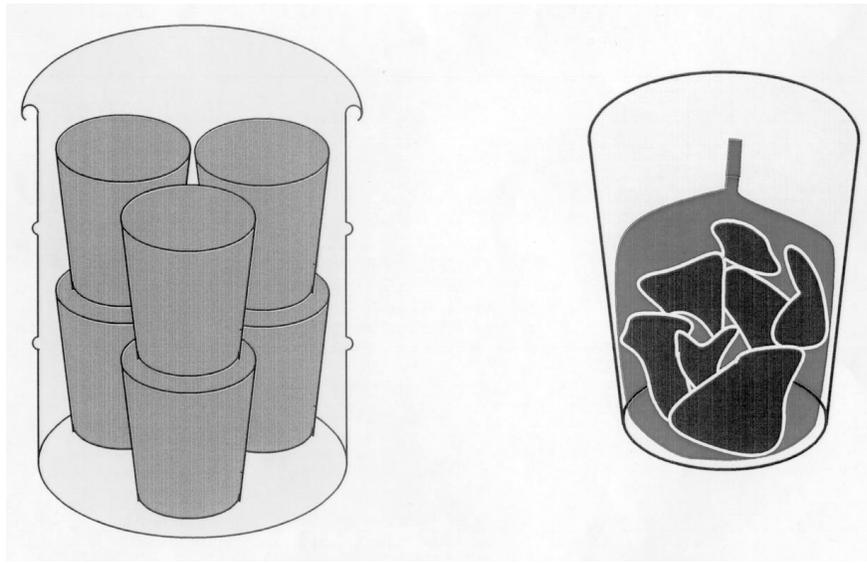
Figure 2. Container for inflammable, partial combustible and incombustible waste. The left sketch shows the 200 L drum with six cardboard boxes inside. The right sketch is an individual cardboard box.
