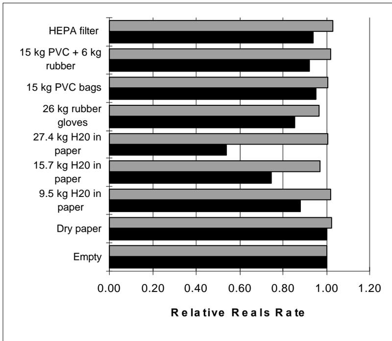
Figure 5. Relative reals rate before and after AAS correction. The dark line is the uncorrected relative reals rate and the light-colored line is the corrected relative reals rate.
