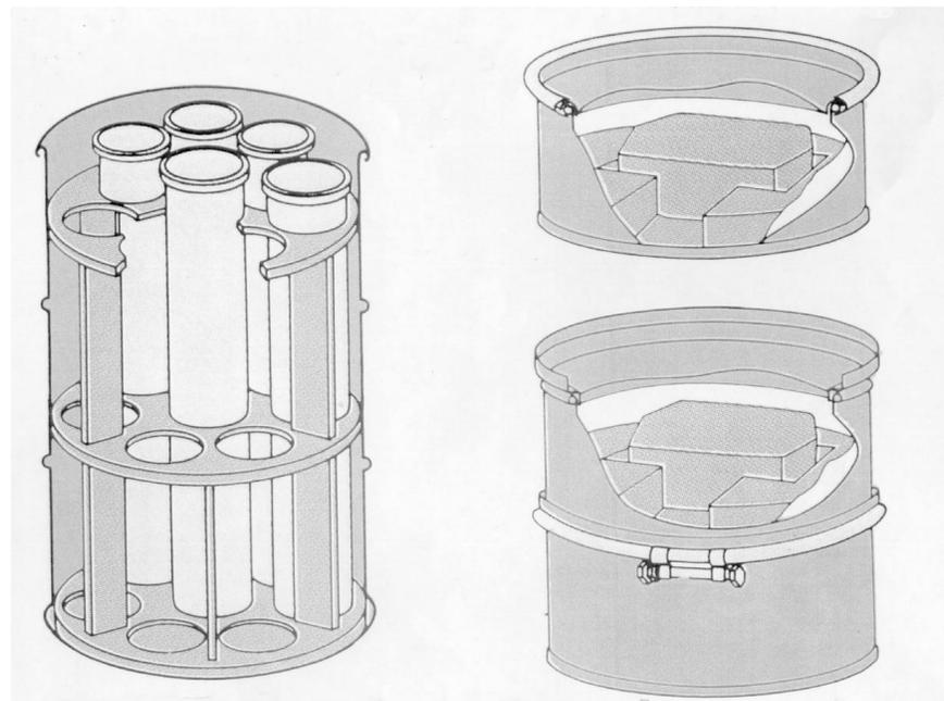
Figure 3. Containers for metal ingots (left sketch) and ceramic-like blocks (right sketch).
